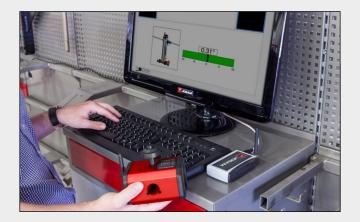
The camera based calibration is an extension for the JOSAM cam-aligner system. Measurements are calculated and displayed in the accompanying software. Reports are printed from the PC.
