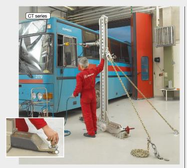
The floor anchoring is exceptional when it comes to repair of minor damage, as for this bus. In this case the cab tower is fixed with a nose bracket directly in the expander hole at the front and with chains at the rear. The tower is pretensioned with an impact wrench. The pulling angle is quickly adjusted sideways and the tower locked into position with a pin.
