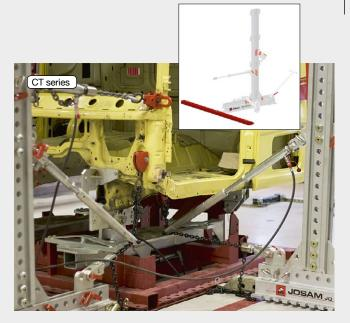
The nose bracket kit allows the trolley to be locked directly to the cab bench for cab repair jobs.
