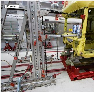
The I-beam system fixes the cab tower into floor beams which have been installed in the shape of a "cab square" or as a complete frame straightening bay.
